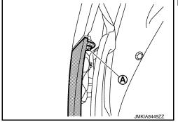
9. Apply protective tape (A) on the part to protect it from damage.
