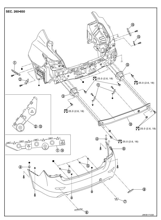
Rear bumper side bracket A LH ② Rear bumper side bracket B LH 1
