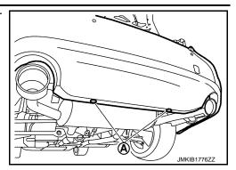
7. Apply protective tape (A) on the part to protect it from damage.
