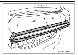
Insert a remover tool (A) between trunk lid molding and trunk lid panel, cut double-sided tape using a cutter (B) while lifting trunk lid molding.
