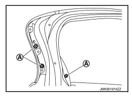
4. Remove rear door sash molding fixing rivets.
