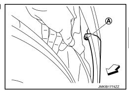
Remove rear bumper fascia assembly fixing screws (A) of bumper lower side (LH and RH).
