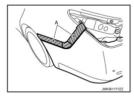
8. Pull rear bumper fascia side toward the vehicle side to disengage the fitting of rear bumper side bracket and rear bumper fascia side according to the numerical order 1→3 as shown by the arrows in the figure.
