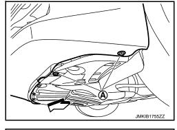
Remove front bumper fascia assembly fixing screws (A) (LH and RH).
