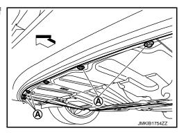
7. Remove fender protector mounting bolts (A) from front side of front fender protector front (LH and RH).
