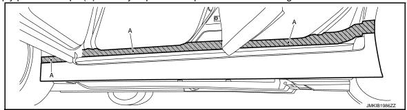
6. Disengage sill cover fixing clips from rear end to front end of vehicle using remover tool (A), and then remove sill cover.
