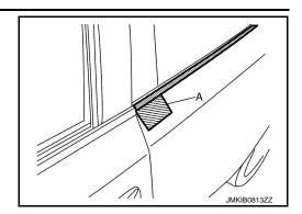
Disengage fixing pawl of rear door outside molding front and rear end, using remover tool (A) and (B).
