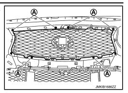
4. Disengage fixing pawls from back side while pulling front grille toward vehicle front, and then remove front grille.
