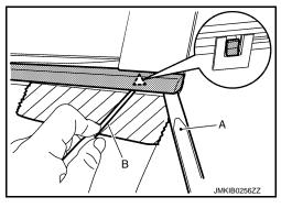
5. Twist front door outside molding toward the direction of the arrow, and then lift up and remove it.
