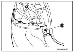
Remove rear bumper fascia assembly fixing screws (A) (LH and RH).
