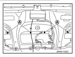
Disengage fixing clips of trunk lid finisher from inside of trunk lid, and then remove trunk lid finisher.
