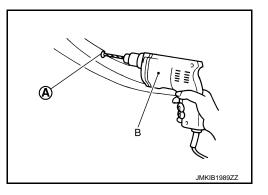
5. Remove rear door sash molding from rear door sash cover fixing pawl, and then remove rear door sash molding.
