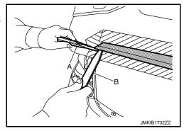
3. Disengage trunk lid molding fixing clips, using a remover tool (A), and then remove trunk lid molding.
