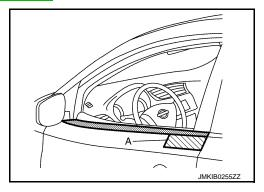
4. Disengage rear end of front door outside molding fixing pawl using remover tool (A) and (B).
