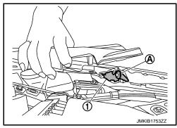
6. Remove front bumper fascia assembly mounting bolts (A) of bumper lower side.
