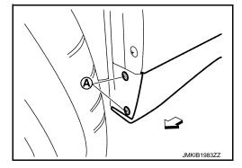
2. Remove sill cover fixing screw (A) and clips (B) of sill cover rear end.
