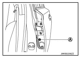
4. Remove rear door sash cover fixing rivets.
