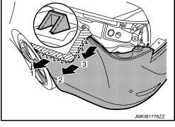
Disengage rear bumper fascia assembly fixing clips as shown by the arrow in the figure
