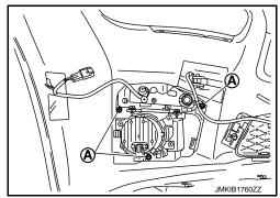
Disengage front bumper finisher fixing pawls, and then remove front bumper finisher (LH and RH) as shown by the arrows in the figure.
